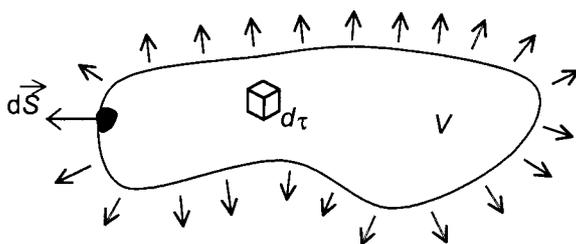
$$F_{\vec{V}}(S(V)) = \iint_{S(V)} \vec{V} \cdot d\vec{S} = \iiint_V \text{div } \vec{V} d\tau$$
