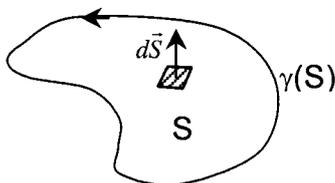
$$C_{\vec{V}}(\gamma(S)) = \iint_S \overrightarrow{\text{rot}} \vec{V} \cdot d\vec{S}$$
